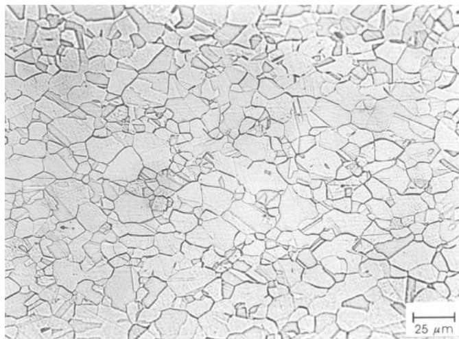
FIG. 1. Characteristic microstructure of a Ni–Al polycrystalline alloy cathode. Light micrograph.
